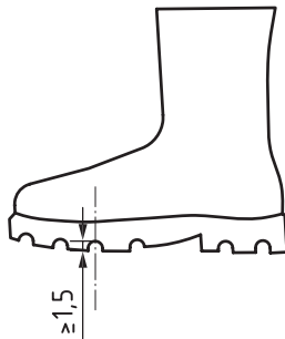
Figure B.1 — Cracks in sole
